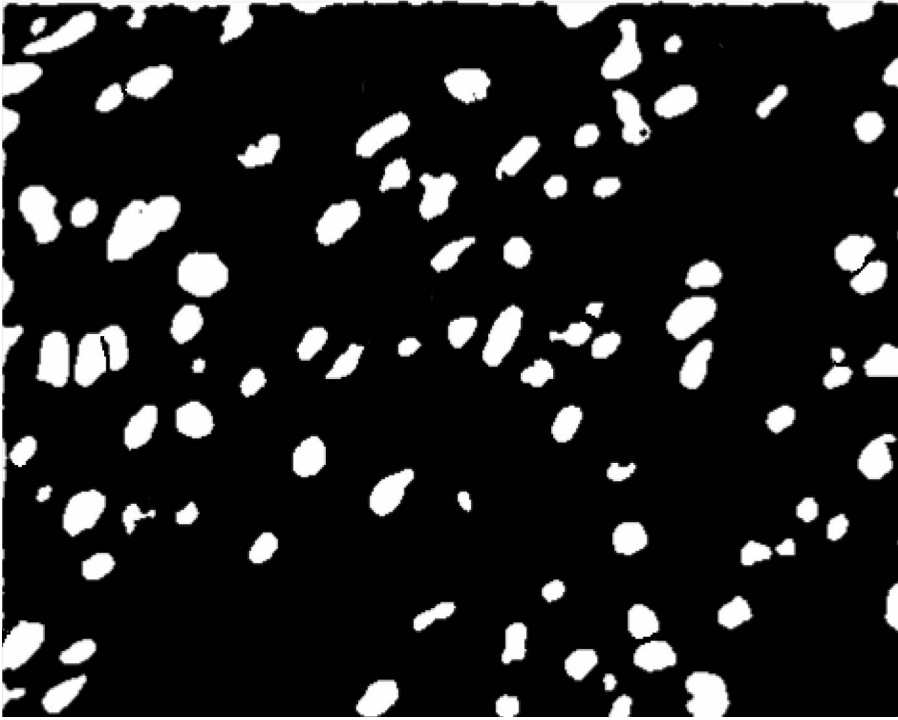
Figure 2. Binary image obtained after applying the unsupervised SVM clustering-based pixel segmentation algorithm.
