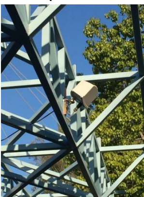
Radar RTMS G4 (Remote Traffic Microwave Sensor)
